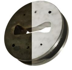
With wet blast technology extruders can achieve a quicker, more effective and consistent polishing action that can improve the die success rate when compared with conventional systems.
